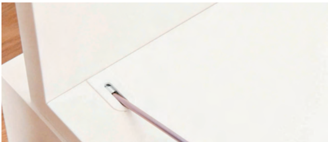
Join furniture elements with cordless drill and Cabineo tool. Easy, fast working with preset torque approx. 2.5 Nm.
